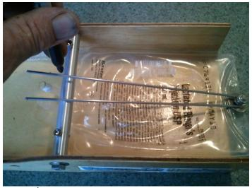
Step 3 \tau Place the bag so that the outlets are behind the bar and mark the wires where they need to be cut as shown. Add 3/4's of an inch to this mark when mounting in short rails.
