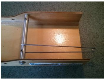
Step 4 ↑ Place one side in bar so that the wire is flush with the back of the bar and tighten the pinch bolt.
